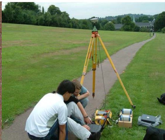
Figure 6: GPS Zero Baseline Trial
