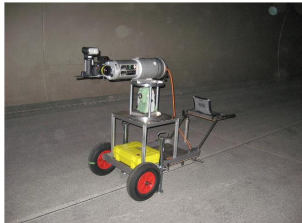
Figure 2. Light metal frame with sensors attached to trolley carrying control computer, WLAN display and power supply
