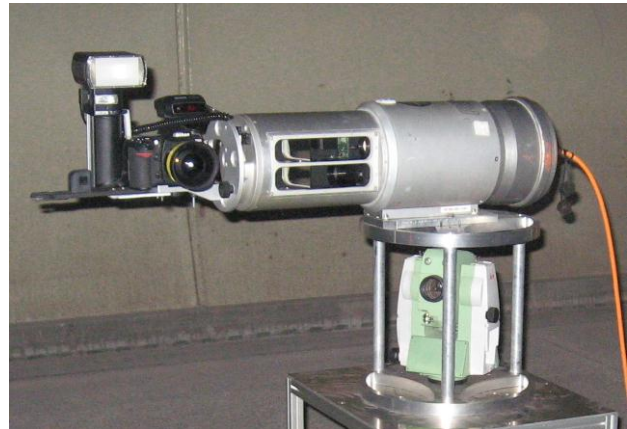
Figure 1. 3-d laserscanner (RIEGL), digital camera (NIKON) and totalstation (LEICA) on light metal frame
