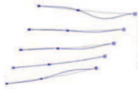
Model 1 - 41 Elements Column Demand: 98.000KN Buckling Load (Capacity): 25.000KN
