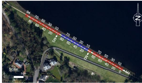
Fig. 5 Non-intrusive ERT arrays (M1, M2 and M3) 96 m long and 2 m electrode spacing covering the whole length of Mugdock dam.
