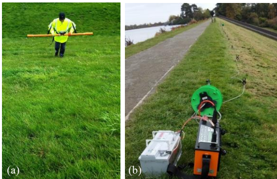
Fig. 4 Non-intrusive geophysical investigation using (a) an EM instrument and (b) ERT arrays installed on the crest of Mugdock reservoir dam.
