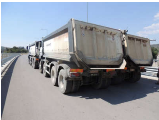
Figure 11. Live load used for testing of bridge B1
