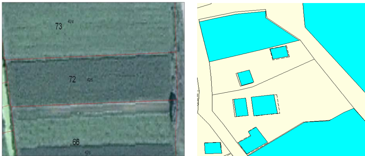
Image 3. The difference between extracted data from satellite image (■) and topographic map that produced by terrestrial surveying(□)
