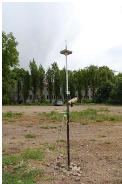
Figure 1. RTK Topcon HyperPro receiver over one of the test marks
