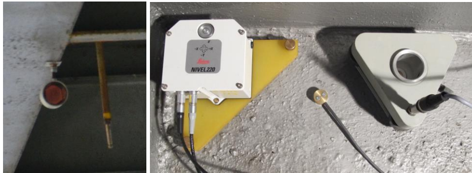
Fig. 6 Stabilization of the measuring points
