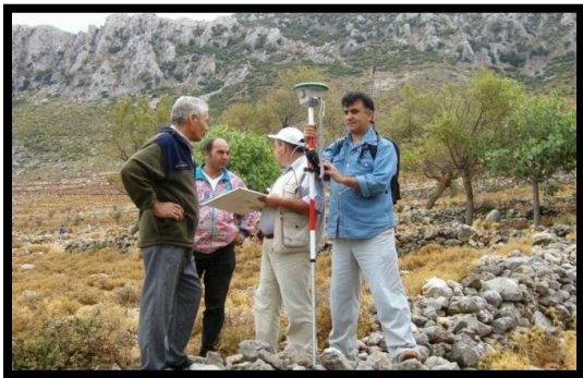
Figure 7. C-Rated Ground Control Point Static GNSS Measurement
