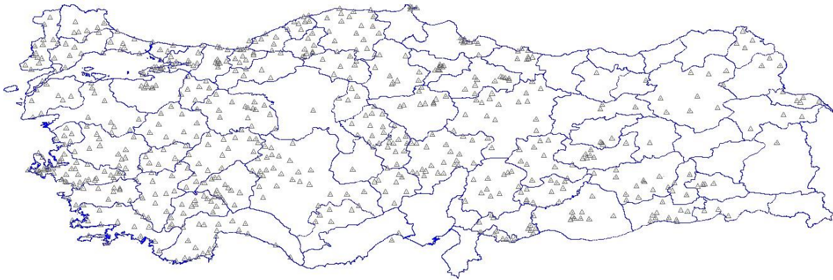
Figure 6. Distribution of 700 Ground Control Points measured by CORS-TR System
