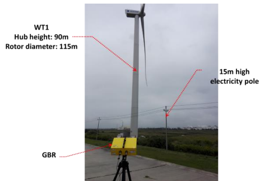
Figure 2: GBR placed orthogonally to WT1
