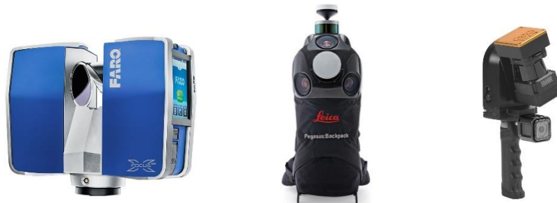
Figure 1: From left to right: FARO Focus3D X330 1 , Leica Pegasus:Backpack 2 , GeoSLAM ZEB-REVO 3
