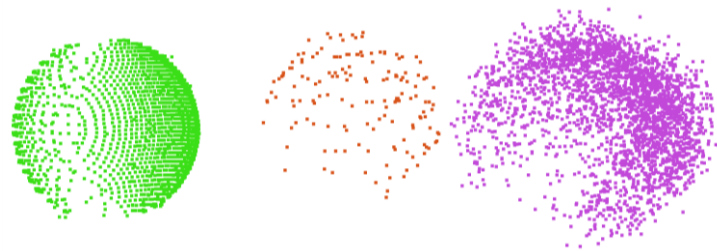
Figure 9: Comparison of a sphere (radius 75 mm) as found in the point clouds available for analysis (from left to right: F3D, LPB, ZEB)
