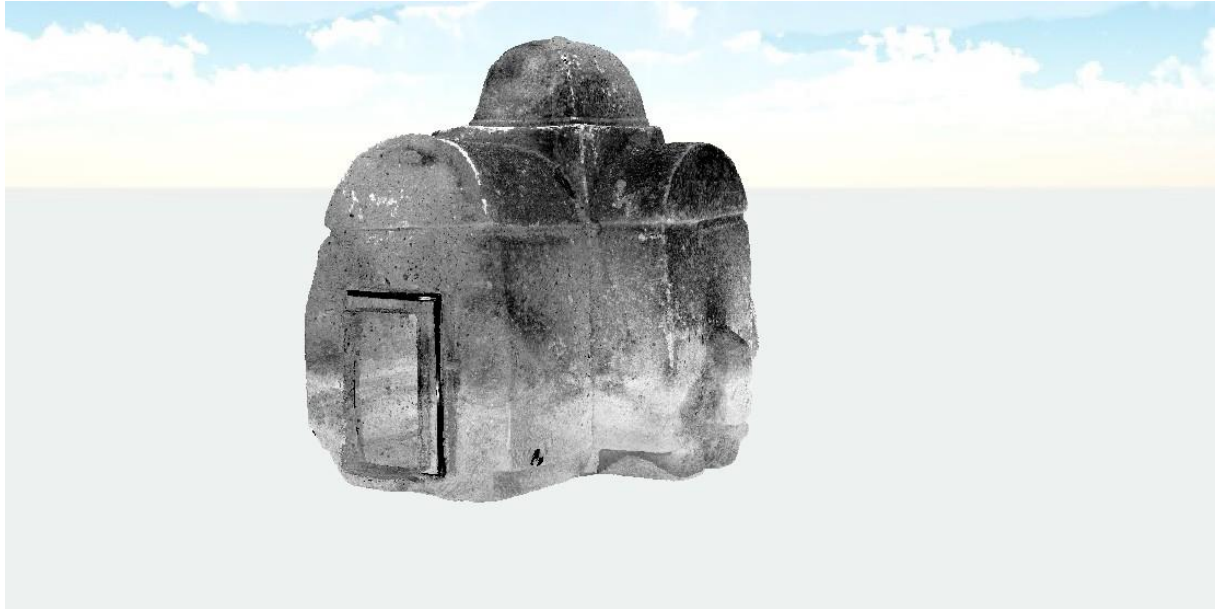
Figure 10. A 3D model of the Cross Church generated with Faro Scene.
