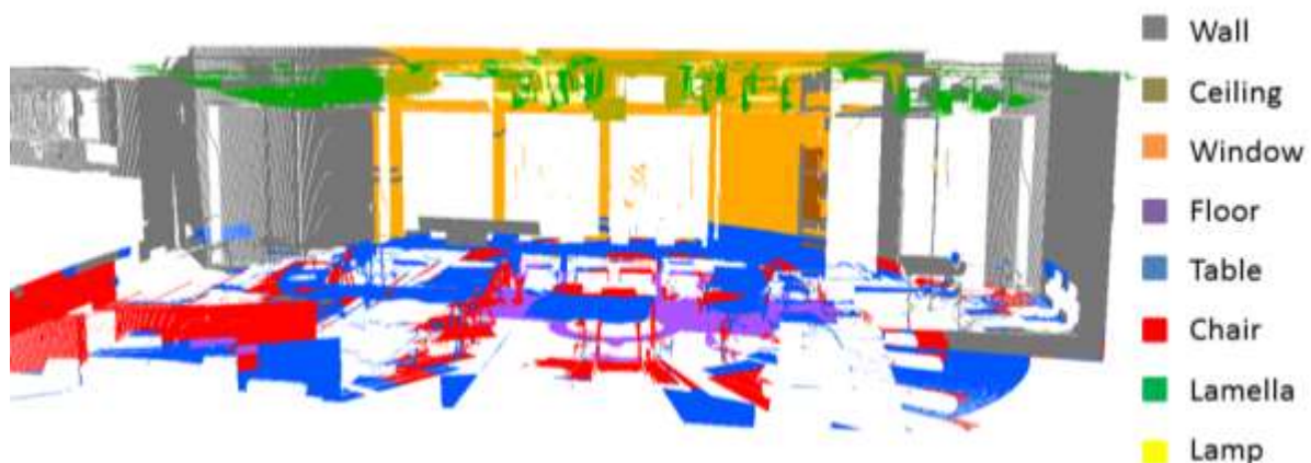
Figure 6: Classified 3D point cloud of an indoor scene. Lecture hall with randomly arranged furniture.
