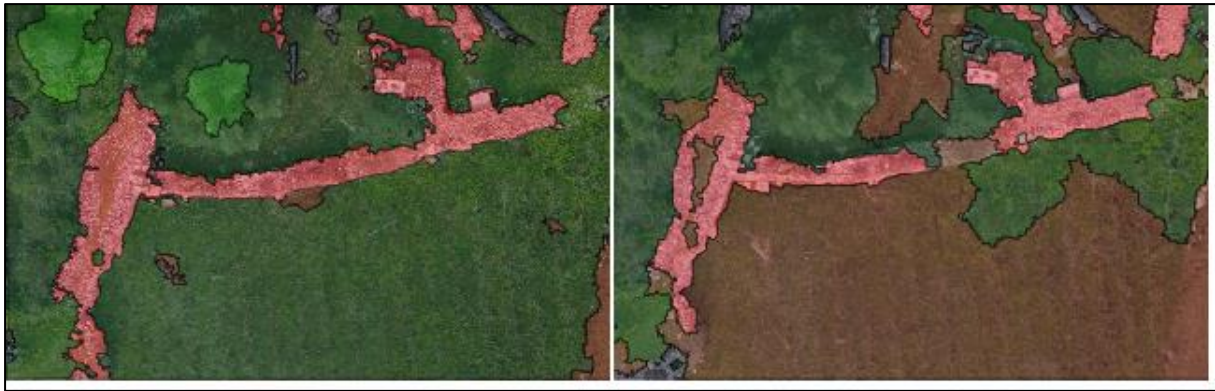
Figure 5 Comparison of classification results of data with higher resolution (left) and lower resolution (right), detail 1
