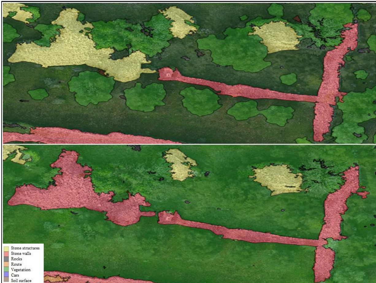
Figure 4 Comparison of point cloud (up) and digital orthophoto maps (down) classification results, detail 2
