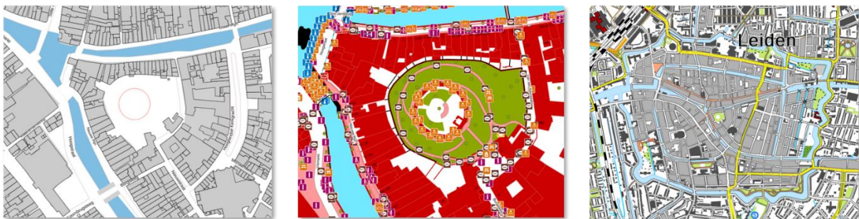
Figure 2 a. Key Register Addresses and Buildings (BAG), b. Key Register Large Scale Topography (BGT), c. Key Register Topography (BRT).
