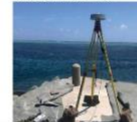
Above and below: Static GNSS Stations as part of the 7 days field survey campaign
