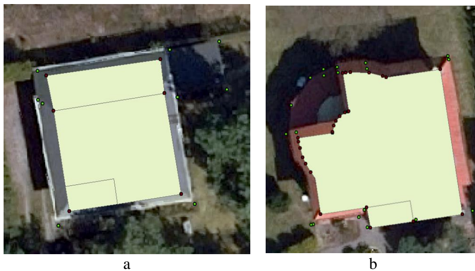
Fig. 6. Errors in building extraction: a - omitted part of the building with roof partially obscured by vegetation; b – a red paved terrace erroneously included as the building roof outline.
