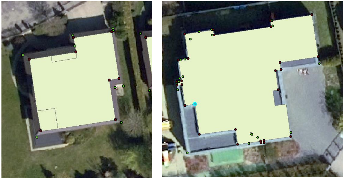
Fig. 5. Correctly delineated outline of the building's roof with a clear offset from the ground survey points marking the ground level.
