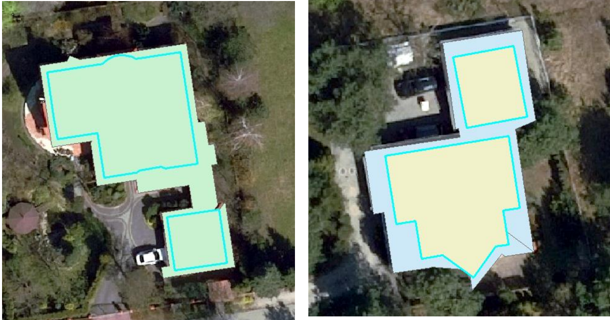
Fig.6. Errors between data in the building registry and buildings extracted from LIDAR data.
