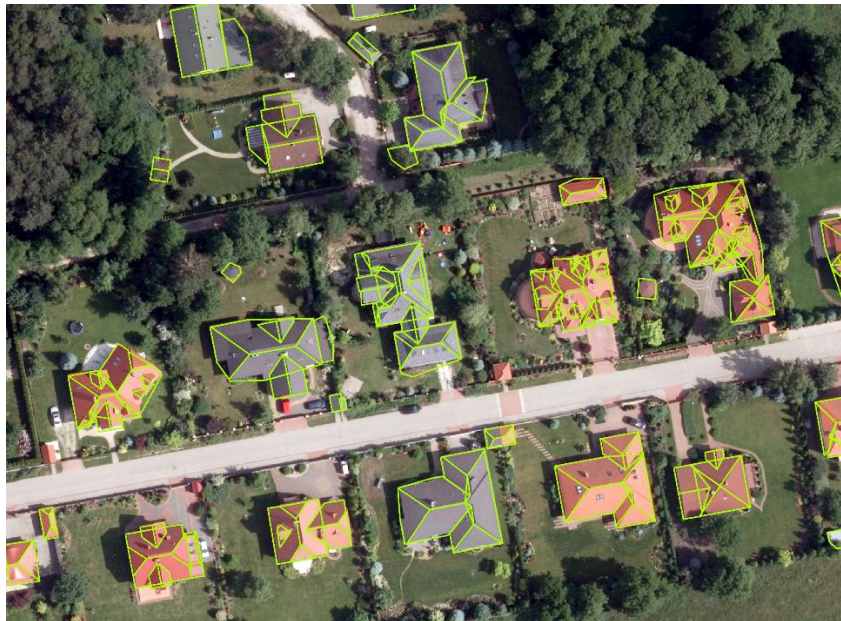
Fig.4. Multi-slope roof patches delineated by ENVI algorithm
