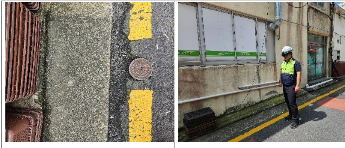
Figure 11 Left: Track markers, manholes, Right: Verifying pipe locations and their real-world counterparts using HoloLens
