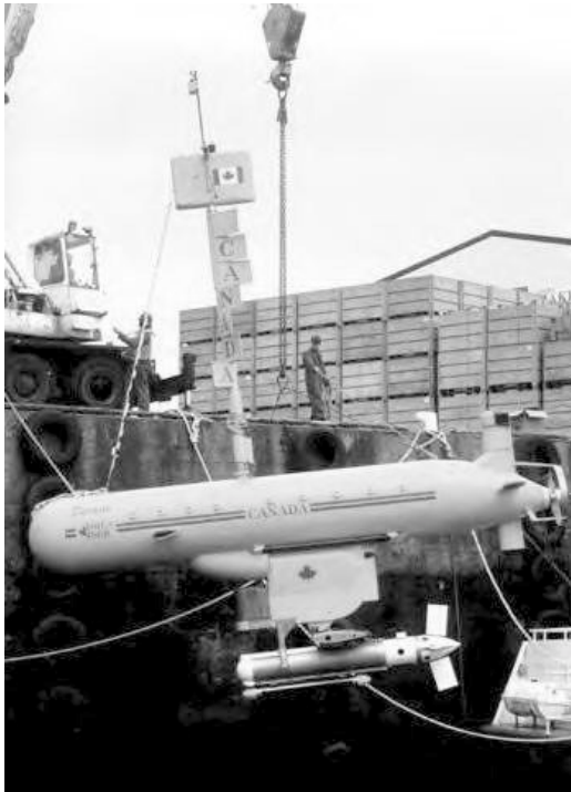
Figure 6: International Submarine Engineering's semi-submersible Dorado AUV with its Aurora towbody
