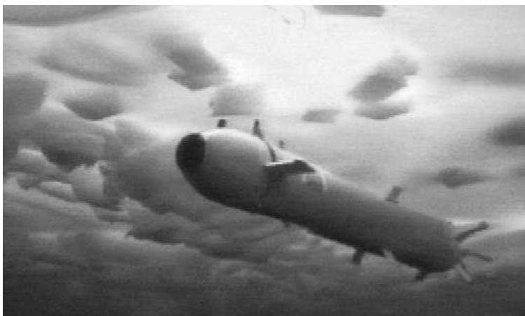
Figure 9: International Submarine Engineering's Theseus cable laying AUV beneath the polar ice
