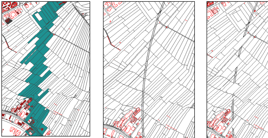
Figure 6: Left: whole parcel is affected, middle: new parcels are generated which results in a parcel pattern reflecting the 2D extent of the 3D object, right: combination of new parcels and parcels that are not divided.
