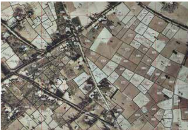
A vectorised field map showing the resulting cadastral map with parcel boundaries in Ethiopia. Image © Zerfu Hailu.
