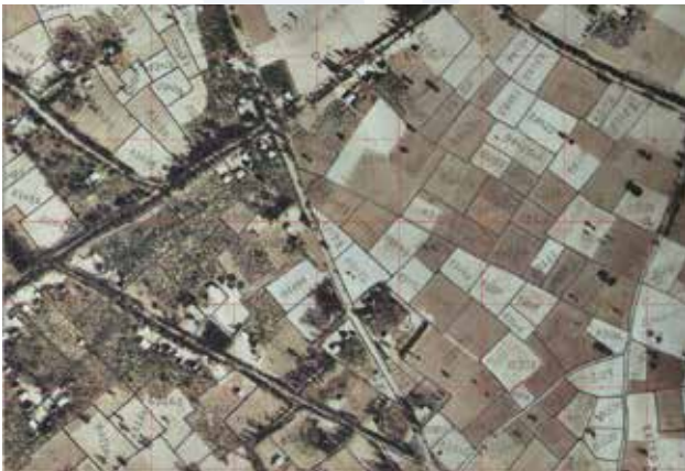
Aerial imagery used as a field work map sheet with a georeferenced grid in Ethiopia. Image © Zerfu Hailu.
