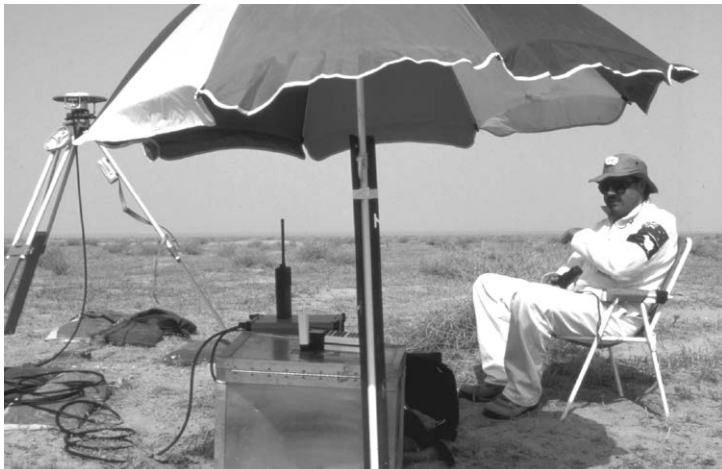
Figure 4: A GPS survey station.
